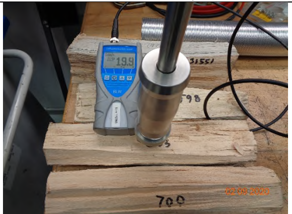
6) Recording of HF fuel load moisture
