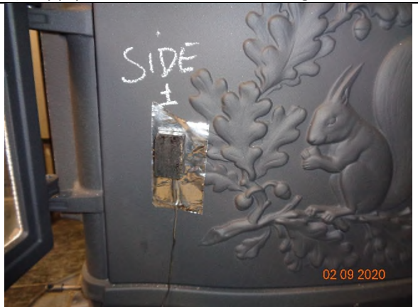
4) Measurement of surface temp (5 in total)
