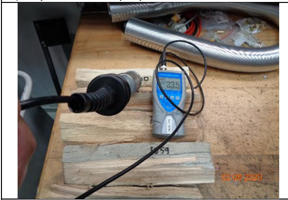
7) Recording of LF fuel load moisture
