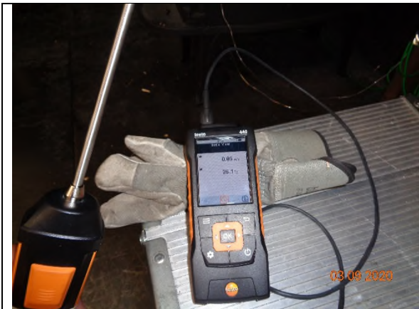
9) Air velocity measurement, end of the MF test
