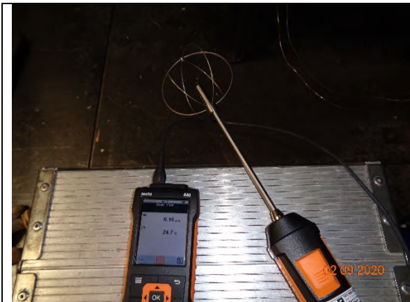
9) Measurement of air velocity prior
