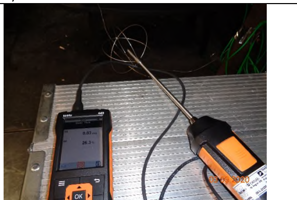
7) Intermediate air velocity measurement
