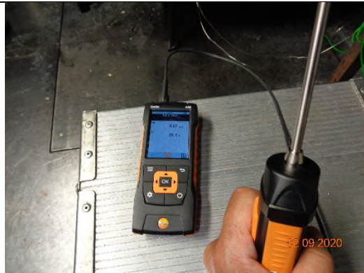
17) Air velocity measurement at the end
