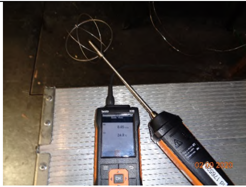
16) Intermediate air velocity measurement
