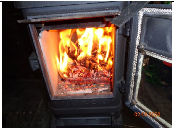
10) Bed of embers at the end of the Cold start
