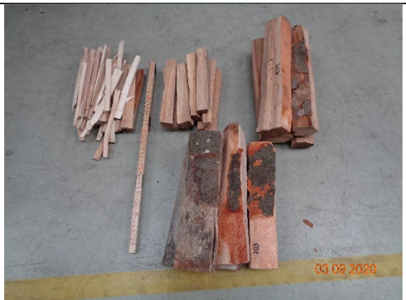
2) Kindling, start-up fuel and HF and MF loads
