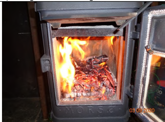
5) Bed of embers at the end of the Cold Start
