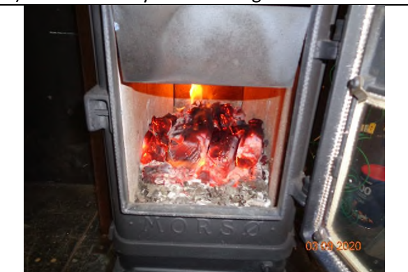
8) Bed of embers at the end of the HF test
