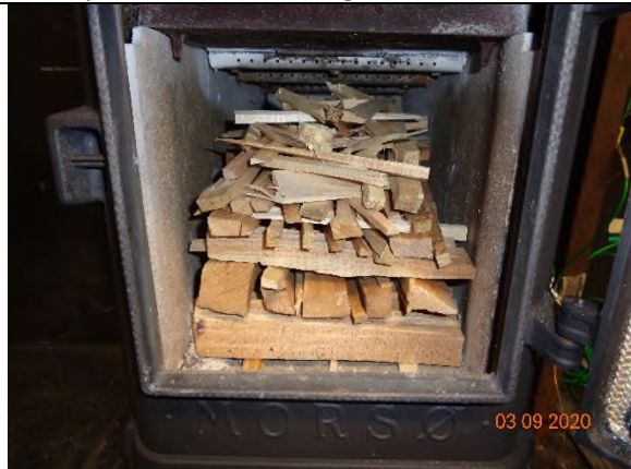
3) Arrangement of kindling and SU fuel
