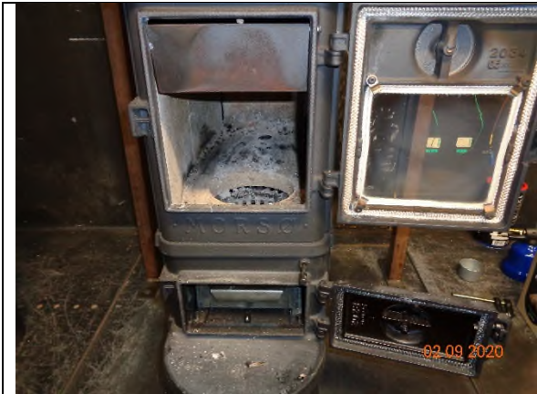
1) Aged 2B Classic 2020 on the test rig
