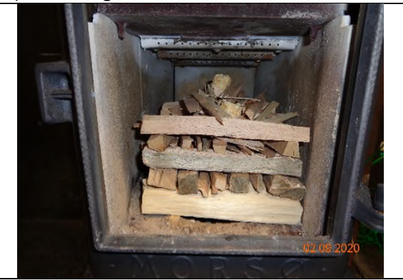
8) Arrangement of kindling and SU fuel
