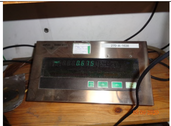
10) Platform scale, end mass of the MF test
