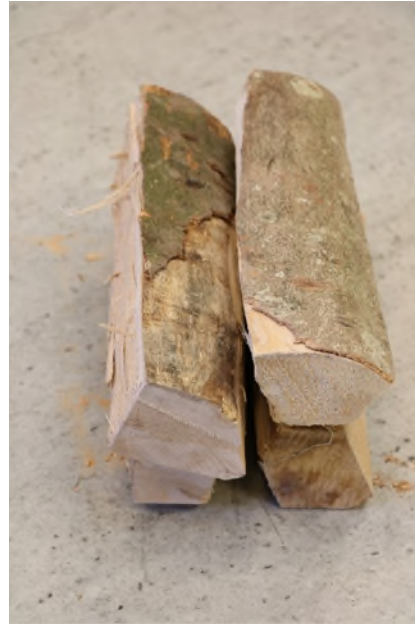
High Fire Load sample Arrangement
