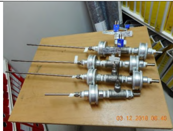
20) Filter holders (Main, 2xSplit and Room)
