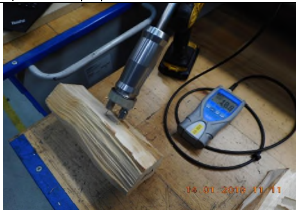
3) Measurement of fuel moisture
