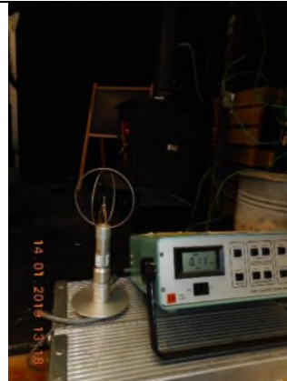
18) Repeated air velocity measurement
